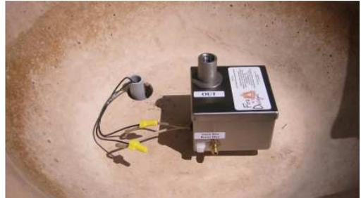
4. On the side of the AWEIS there are two connections for the Pilot Burner Assembly as shown in the photo at right. The white 'quick connect' is the electrical connection and the brass plumbing fitting is the gas connection. There is a label next to these connections, "Attach Pilot Burner Here".
