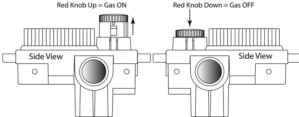
**Fig. 5** E-Stop Gas Timer red knob positions
